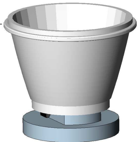
Figure 4. Extending and retracting the large reflector by 13 mm changes the illumination pattern from narrow beam to wide flood pattern. The heat-sink/pedestal (blue part) is part of the lamp, and is not provided by Fraen Corporation.
